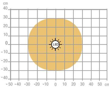
Measurement in Lux on the worktop in profile view at 35 cm:
